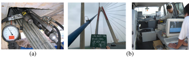
Fig. 1. Direct and indirect methods used to determine the tension force in Vietnam. (a) Load cell, (b) vibration measurement.
