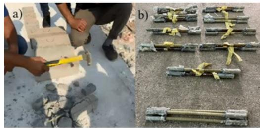
Fig. 3. (a) GFRP bar extraction after burning from prism section, (b) GFRP bar preparation for the tensile test.
