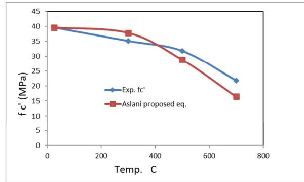
Fig. 7. Burning temperature versus compressive strength (f'c).
