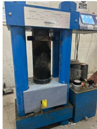
Fig. 8. Compressive strength test.
