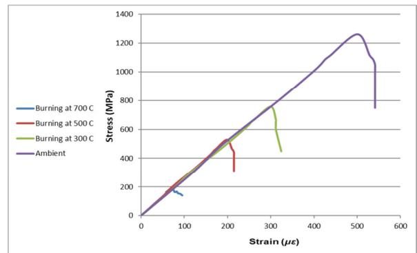
Fig. 11. Stress-strain relationship of burned uncovered GFRP bars.
