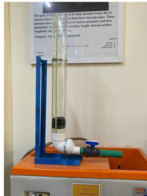
Fig. 2. Laboratory device used for permeability measurement.
