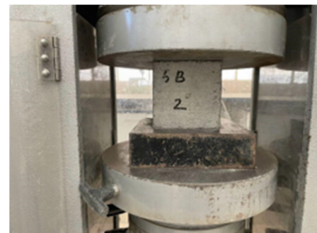
Fig. 3. Specimen under compressive strength test.
