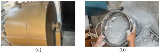
Fig. 2. (a) Grinding and (b) sieving of foam concrete waste.
