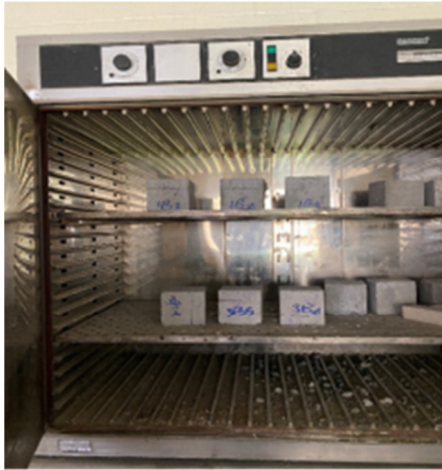
Fig. 7. Cube specimens in the oven.
