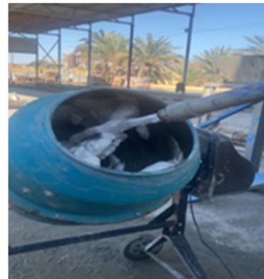
Fig. 1. Preparation of the foaming agent.
