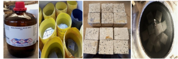
Fig. 6. Sulphuric acid immersion and durability test.
