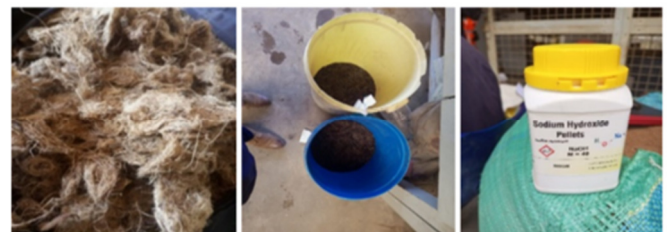
Fig. 3. Treatment of RF with NaOH.
