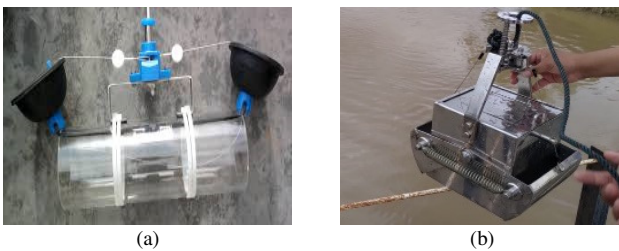
Fig. 2. (a) Van Dorn bottle sampler, (b) Grab sampler.
