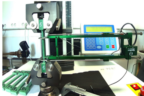
Fig. 6. Specimen subjected to the tensile test.
