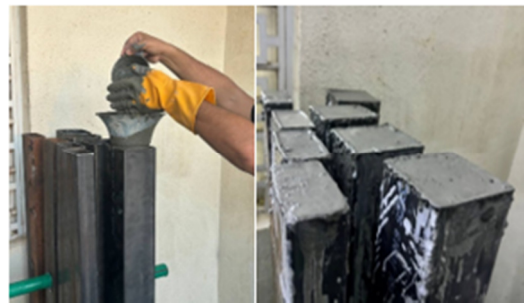
Fig. 1. The casting process of CFST.
