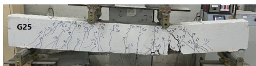
Fig. 13. Cracks at the failure of the G25 beam.
