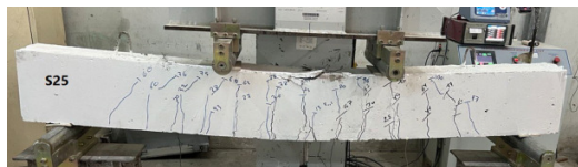
Fig. 12. Cracks at the failure of the S25 beam.
