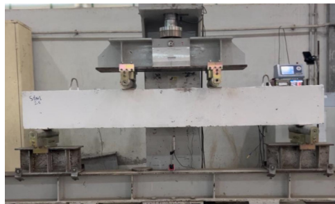
Fig. 8. Beam test setup.
