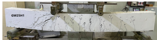
Fig. 16. Cracks at the failure of the GW25H1 beam.
