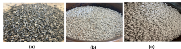
Fig. 1. The three types of LWAs after crushing and sieving: (a) LECA, (b) Ponza, and (c) Thermostone
