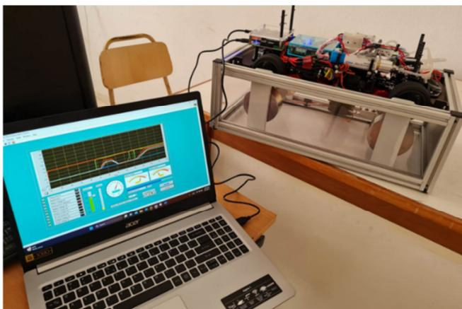
Fig. 5. Bench experiment of the HFCEV in the laboratory.
