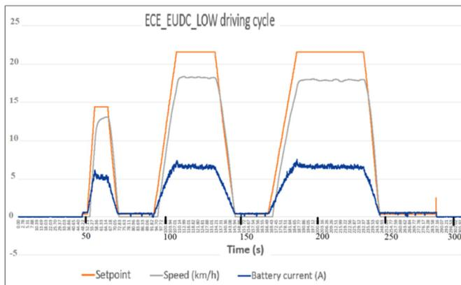
Fig. 11. Real test for European drive cycle output.
