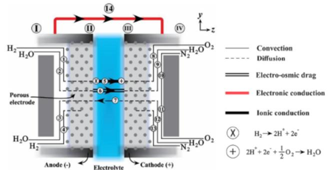
Fig. 2. The schematic of a PEM cell model.
