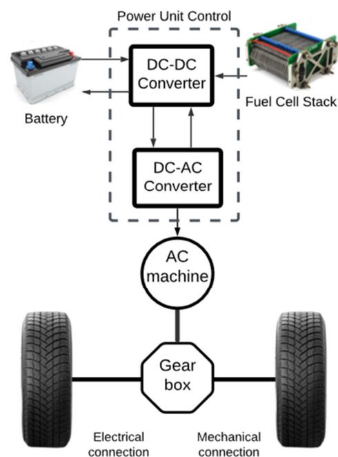
Fig. 1. FCHEV Power train configuration.
