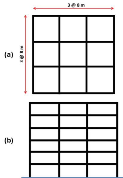
Fig. 1. The layout and design parameters of the building: (a) building plan, (b) building elevation.
