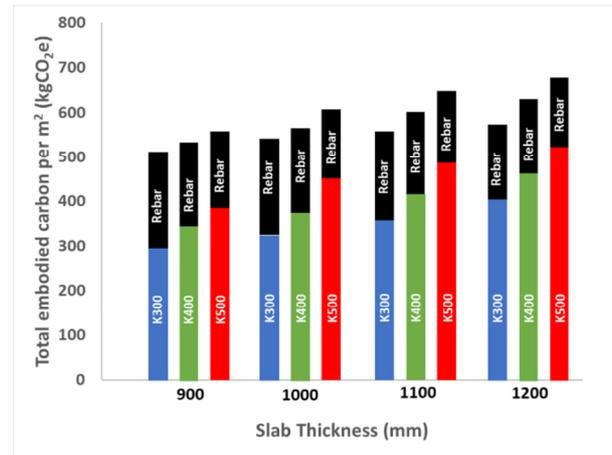
Fig. 2. Total embodied carbon per m<sup>2</sup> of the raft foundation (kg CO<sub>2</sub>e) by material type for varying slab thicknesses and concrete grades.
