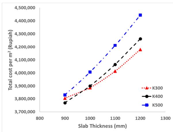
Fig. 4. Total cost of raft foundation across different slab thicknesses and concrete grades.
