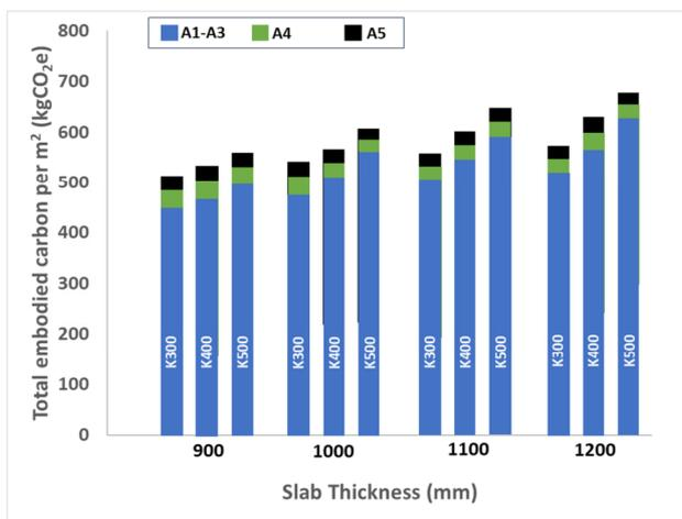
Fig. 3. Total embodied carbon per m<sup>2</sup> of the life cycle stages (A1-A5) of raft foundation (kg CO<sub>2</sub>e) for varying slab thicknesses and concrete grades.
