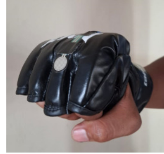
Fig. 3. Glove with FSR 402 implanted inside.
