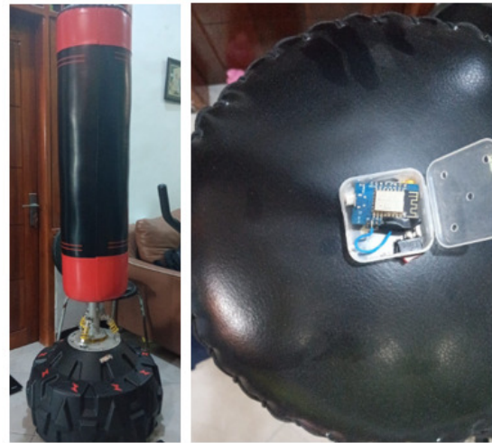
Fig. 4. Punching bag with GY 6500 MPU6500 implanted on its top.
