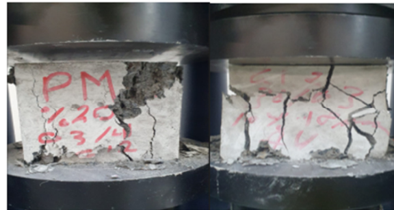
Fig. 7. Failure mode of concrete cubes under compressive test with 20 % powder substitution and 10% CH substitution at the age of 28 days.
