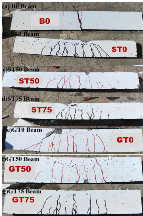
Fig. 13. Mode failure pattern of the tested beams.
