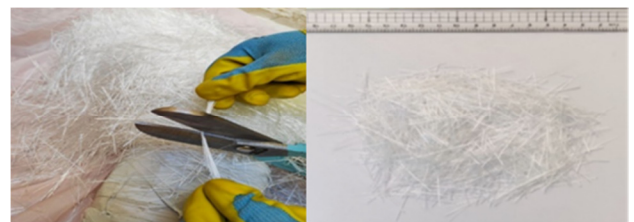
Fig. 4. The process of cutting GF to the required length.
