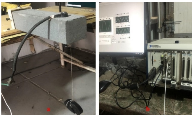
Fig. 4. (a) Damping test setup. (b) Measurement equipment and the LabVIEW system.
