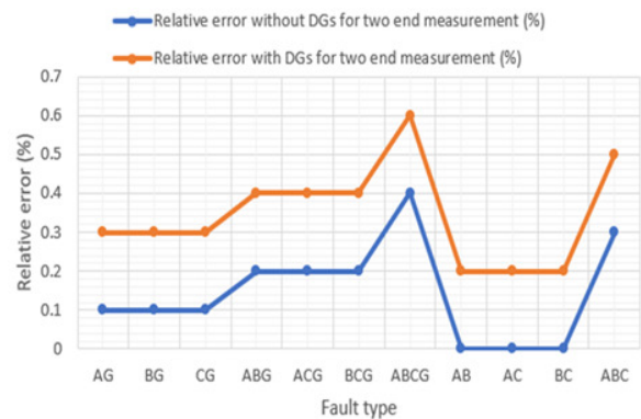
Fig. 15. Comparison of relative error with and without DGs for two end measurement.
