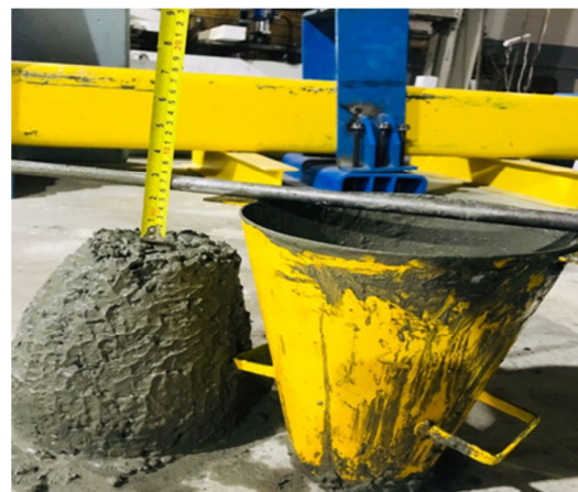
Fig. 5. Slump of 100% RCA replacement ratio concrete mixture test.
