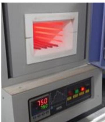
Fig. 2. Muffle furnace used for heating the specimens.
