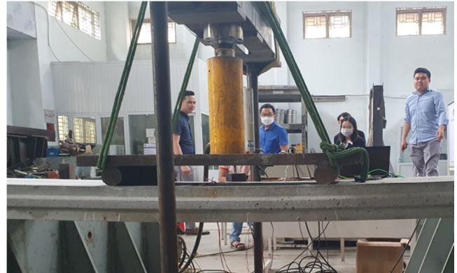
Fig. 2. Actual image of the sample showing deflection and cracking under bending.
