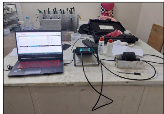
Fig. 4. UPV test setup with asphalt concrete mixes.
