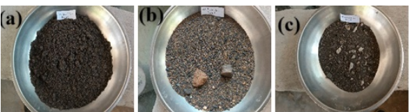
Fig. 2. BA sample from (a) PLTU AA, (b) PLTU PP, and (c) PLTU BK.
