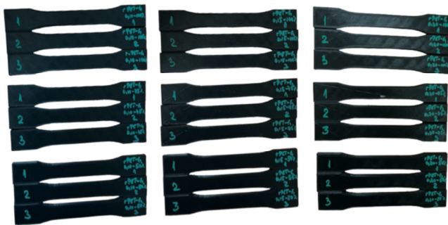
Fig. 4. The rPETG tensile test specimens were fabricated via FDM using an Anycubic 4 Max Pro 2.0 3D printer.
