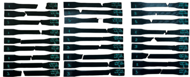
Fig. 6. The rPETG specimens after the tensile test.
