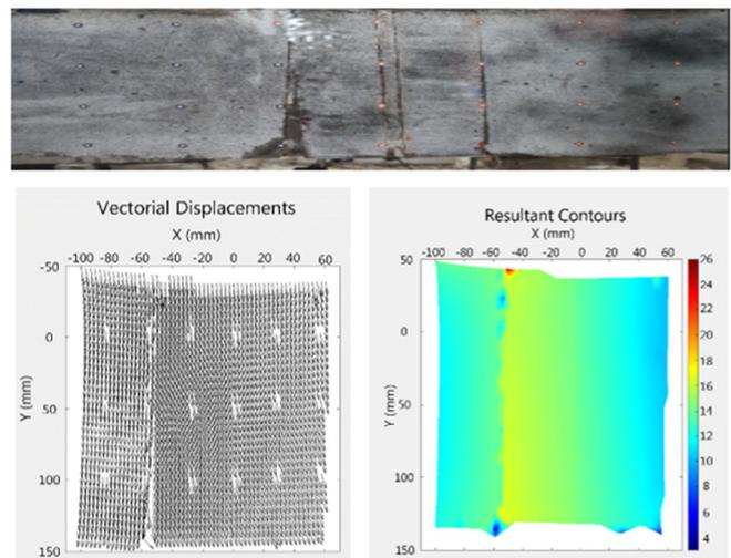
Fig. 7. Particle image processing of ZZ-2 using GeoPIV-RG.
