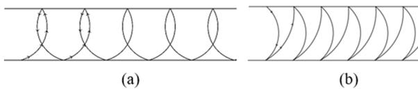
Fig. 2. Welding type: (a) Circular and (b) zig-zag.
