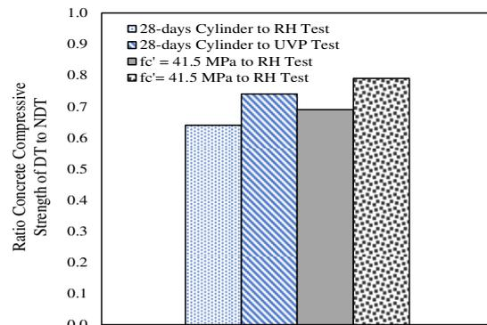
Fig. 4. Ratio of concrete compressive strength based on NDT to DT comparison.
