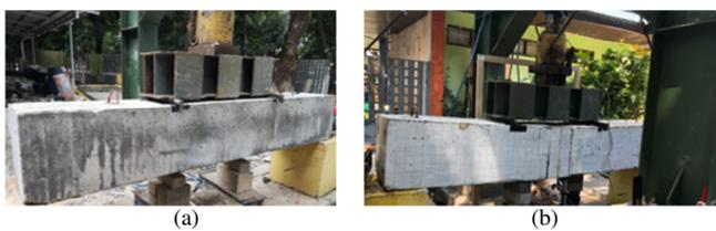
Fig. 5. Flexural strength test: (a) monolithic pile and (b) welded pile.
