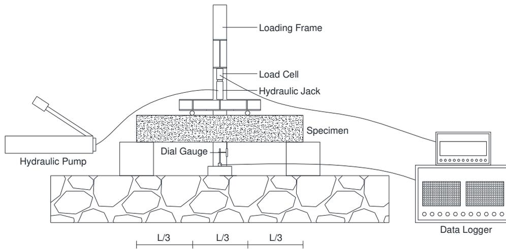
Fig. 3. Flexural strength test set up.
