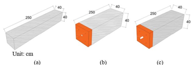
Fig. 1. Industrial concrete pile specimen: (a) Monolithic, (b) female, and (c) male.
