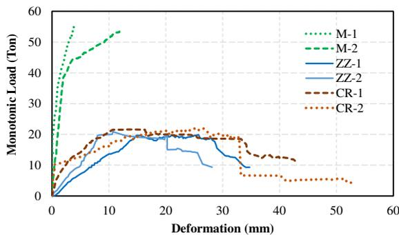
Fig. 6. Monolithic pile and welded pile flexural capacity under monotonic load.
