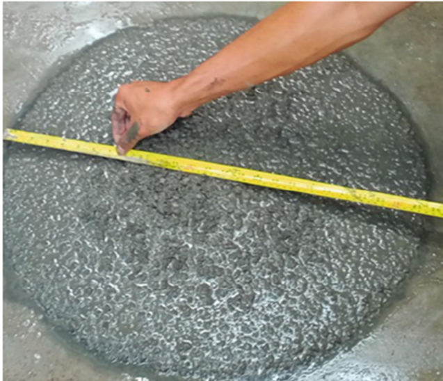
Fig. 1. Slump flow test.
