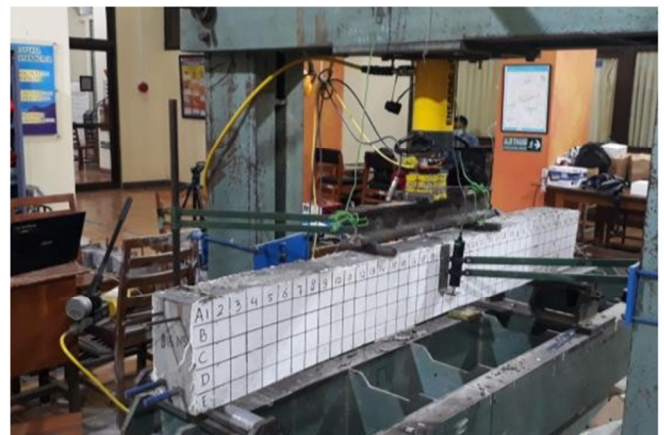
Fig. 3. Setup of beam specimen.
