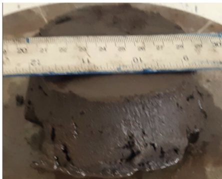
Fig. 3. Flow of geopolymer mortar at 6 M concentration.
