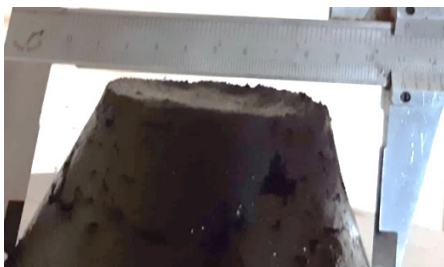
Fig. 4. Flow of geopolymer mortar at 12 M concentration.
