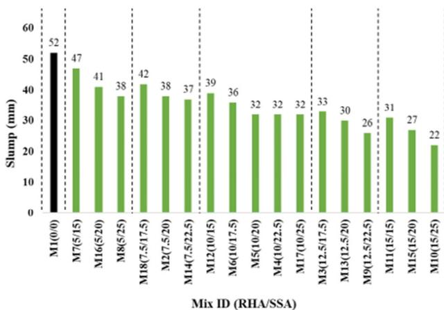
Fig. 2. Slump test results.
