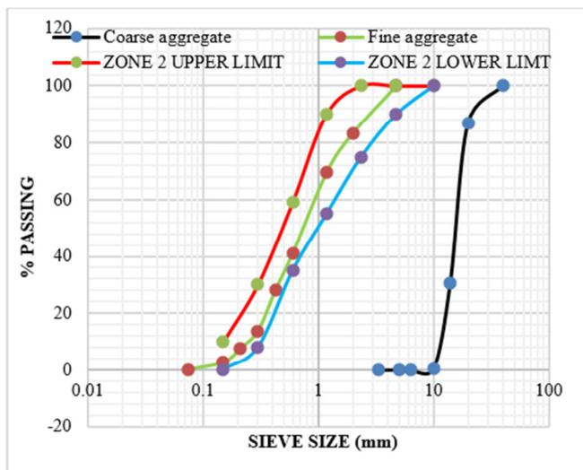
Fig. 1. Particle size distribution of aggregates.
