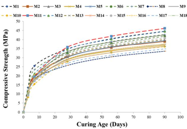
Fig. 4. Compressive Strength vs Age of Curing.
