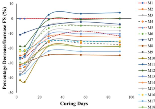
Fig. 7. The rate of RHA concrete Flexural strength enhancement compared to the control (M1).
