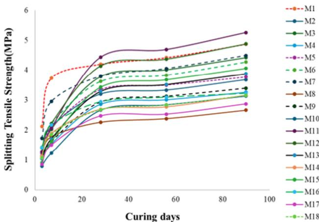
Fig. 8. Splitting tensile strength vs age of curing.
