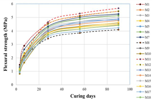
Fig. 6. Flexural strength vs age of curing.
