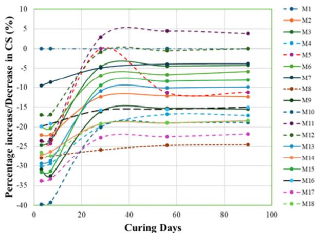
Fig. 5. The rate of RHA concrete compressive strength enhancement compared to the control (M1).
