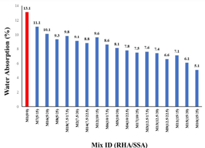
Fig. 10. Water absorption results.
