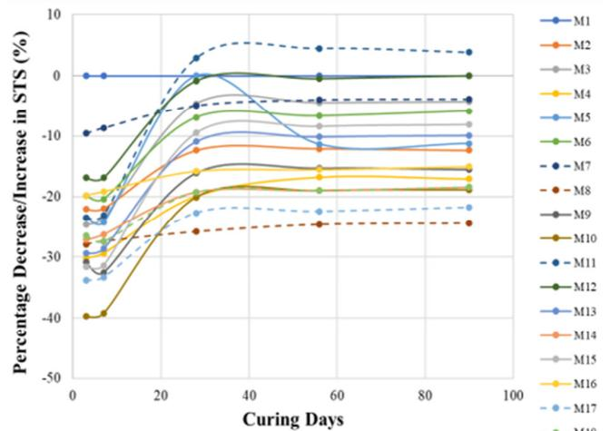
Fig. 9. The rate of RHA concrete tensile splitting strength enhancement compared to the control (M1).
