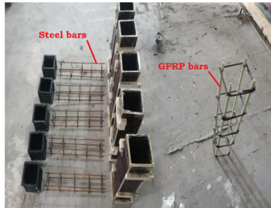
Fig. 2. Wood molds and reinforcing cages.
