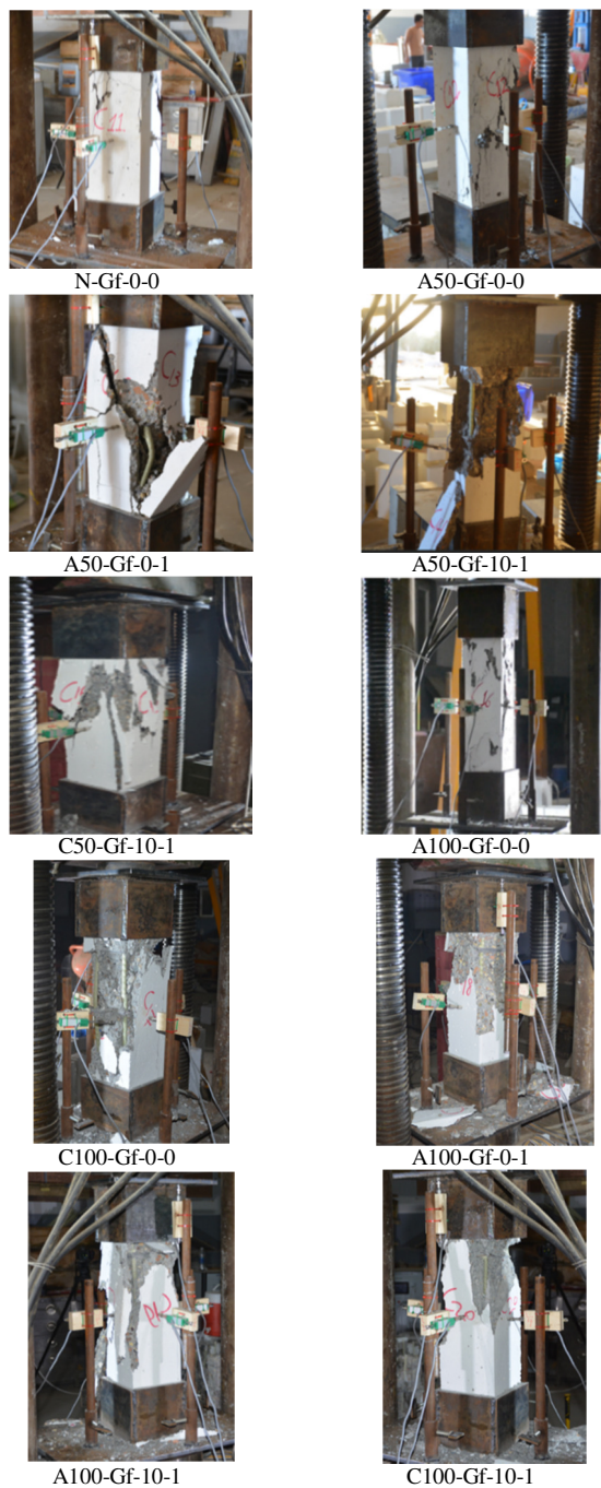
Fig. 20. Failure modes of columns containing GFRP bars.
