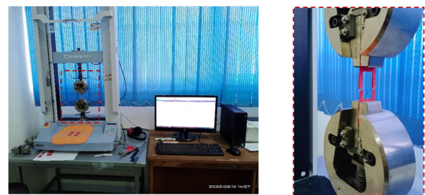
Fig. 2. Tensile strength test of single fiber.
