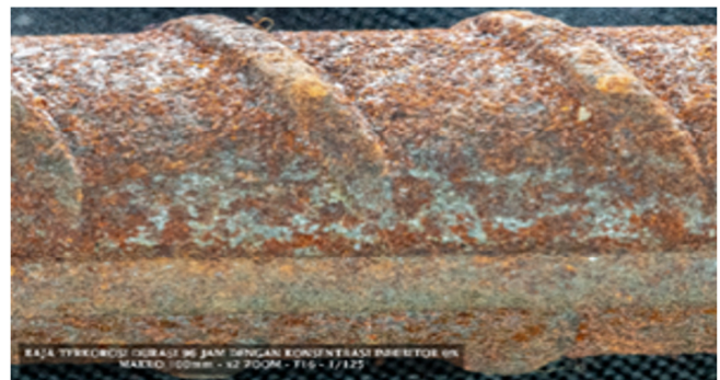
Fig. 10. The 0% concentration steel at 96 hours immersion.
