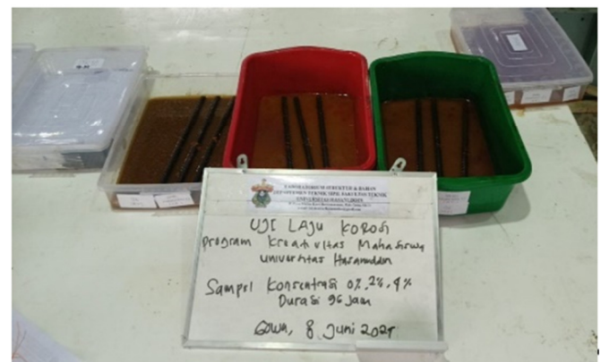
Fig. 3. Corrosion rate and inhibition efficiency test.
