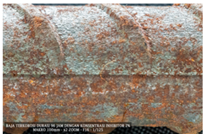
Fig. 11. The 2% concentration steel at 96 hours of immersion.
