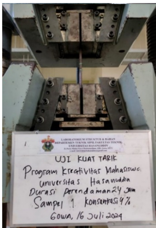
Fig. 4. Steel tensile strength test.
