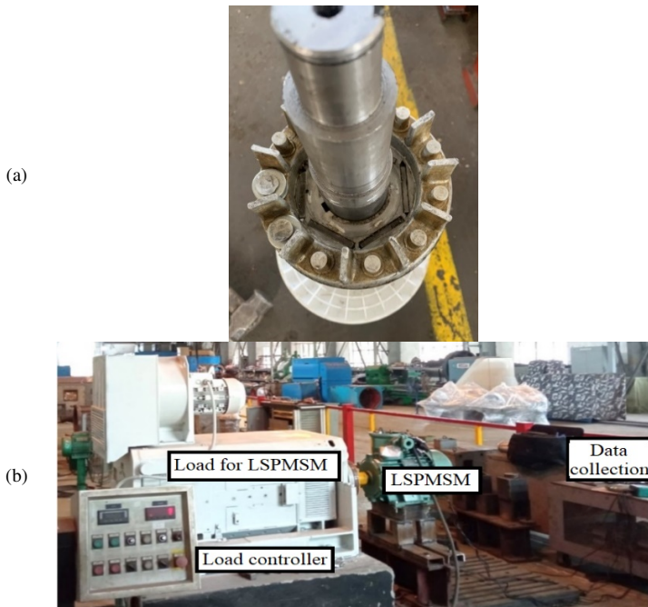
Fig. 10. Test model for performing the experiments. (a) Fabricated rotor and (b) complete system.
