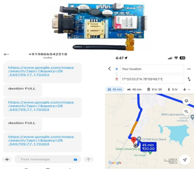
Fig. 7. Send SMS and google map for smart dustbin location using SIM900A.
