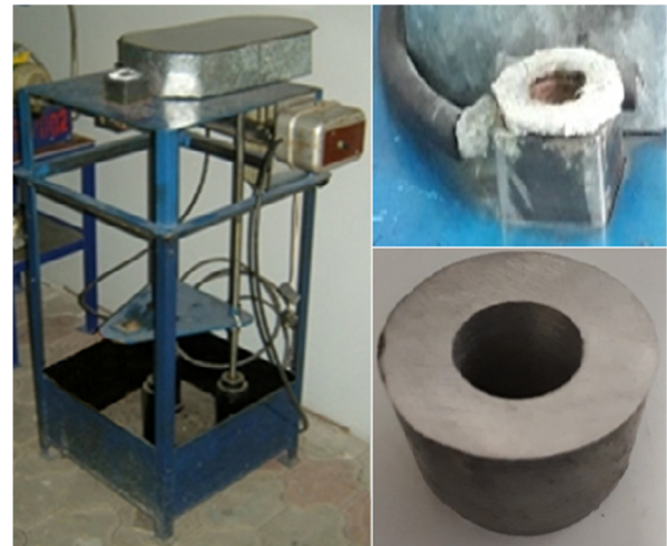
Fig. 1. Facility for continuous casting of billets at the laboratory of Toraighyrov University and hollow aluminum billet.
