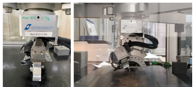
Fig. 7. Residual stress measurement using XRD.
