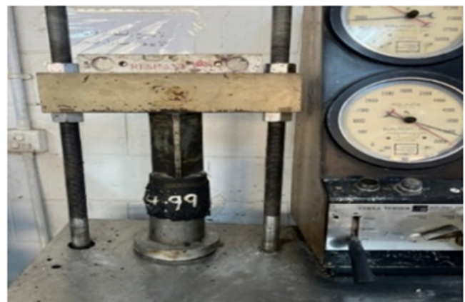
Fig. 7. Testing of compressive strength.
