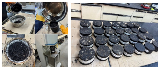
Fig. 4. Preparation of Marshall specimens.
