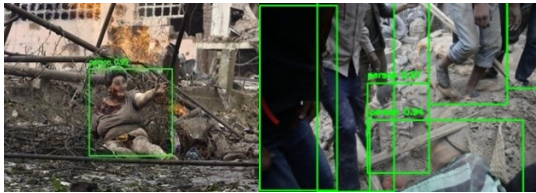
Fig. 5. Detection of human bodies under disaster conditions even with other noisy human objects.
