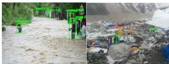
Fig. 7. Different natural disaster locations - human body detection in flood zones and snowy regions.
