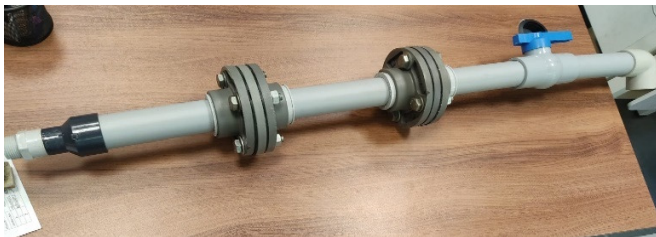
Fig. 3. Two Orifice flanges were connected in series with different orifice-plate patterns.
