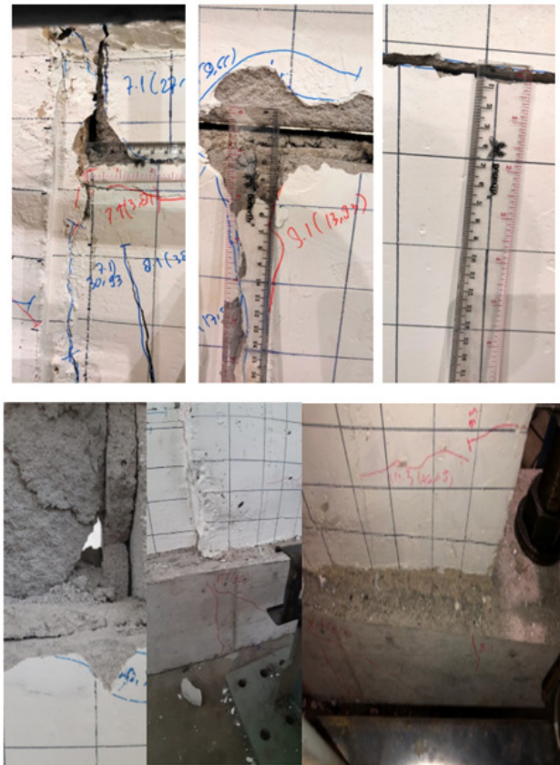
Fig. 11. Failure mechanism in joints between CLC materials of DB-2 specimen.
