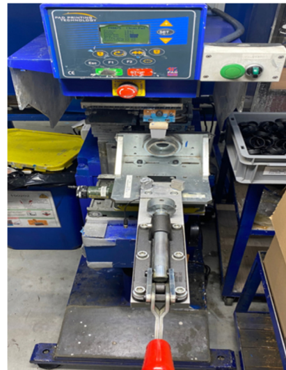
Fig. 3. The current fixture with the clamping device mounted on the pad printing machine.
