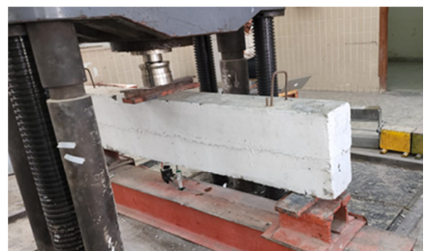
Fig. 6. Composite beams test setup.
