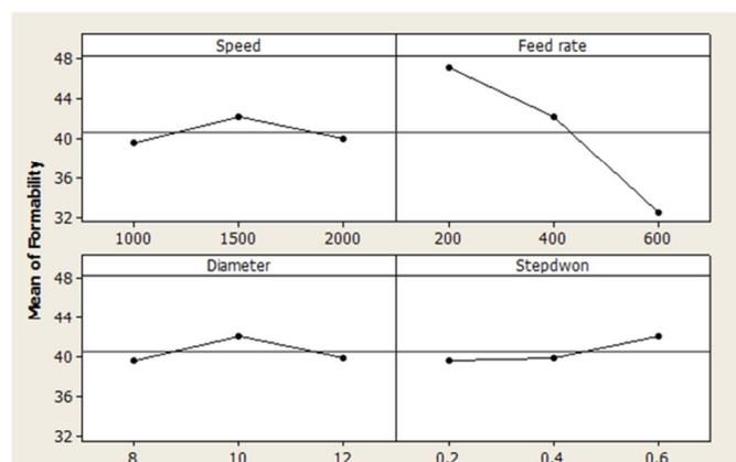
Fig. 6. Mean effect diagram formability.
