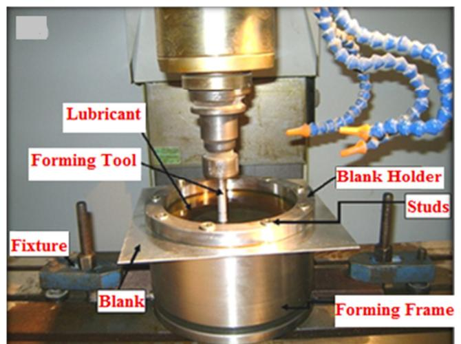
Fig. 2. Conventional CNC milling machine c-tek technology corporation (KM-80 D) experimental setup (die and blank holder).
