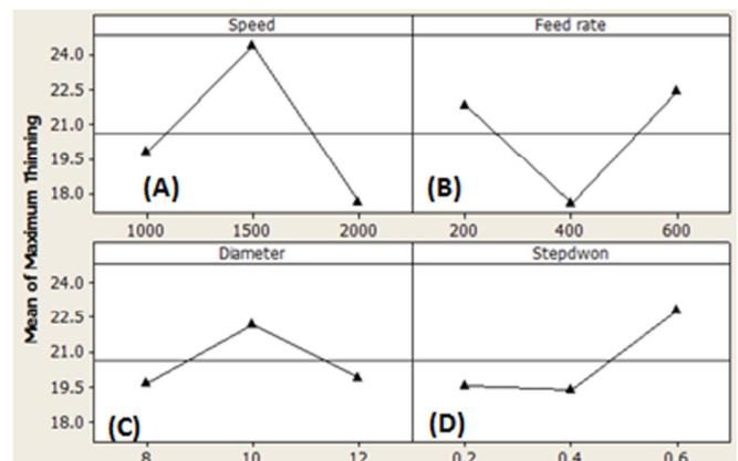
Fig. 5. Mean effect diagram maximum thinning.
