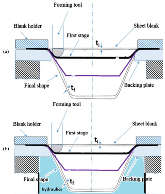
Fig. 1. (a) without hydraulics, (b) with hydraulics.
