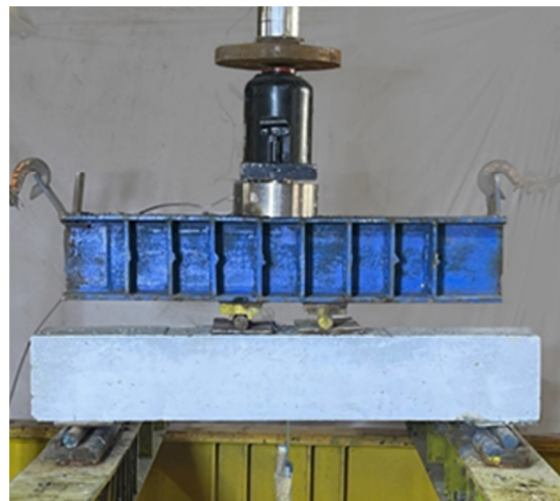
Fig. 1. Loading configurations of the tested beams.
