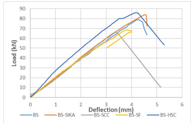
Fig. 6. Effect of the type of new concrete on the load-deflection curves.
