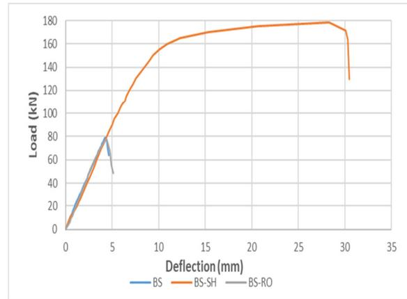
Fig. 8. Effect of the type of bonding method and surface roughness on the load-deflection curves.
