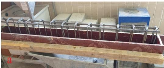
Fig. 2. The wooden mold and reinforcing steel cage for composite beams.
