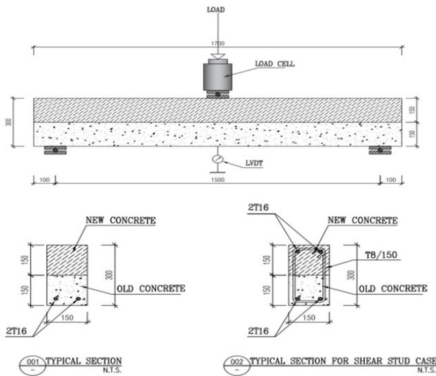
Fig. 1. Details of composite beams.
