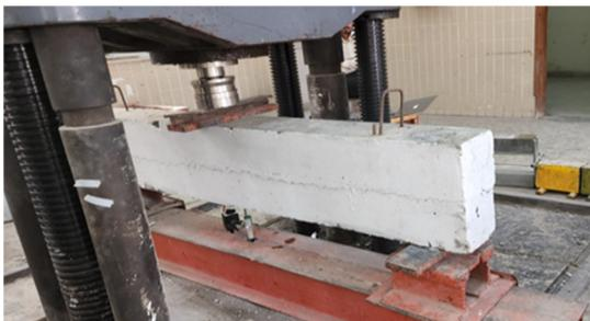
Fig. 4. Composite beams test setup.
