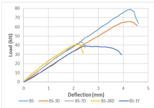
Fig. 5. Effect of old concrete age on the load-deflection curves.
