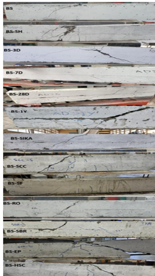
Fig. 9. Failure modes of beams under static loads.
