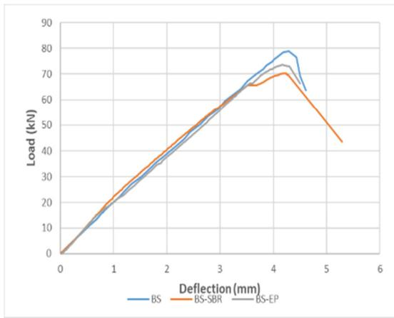
Fig. 7. Effect of the type bonding agent on the load-deflection curves.
