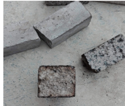
Fig. 6. Black pores in concrete specimens with PBW aggregate after exposure to high temperatures.
