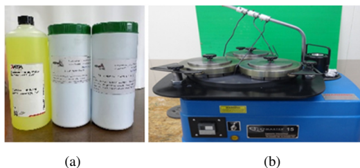
Fig. 2. (a) Alumina ( \text{Al}_2\text{O}_3 ) powder, (b) lapping machine.
