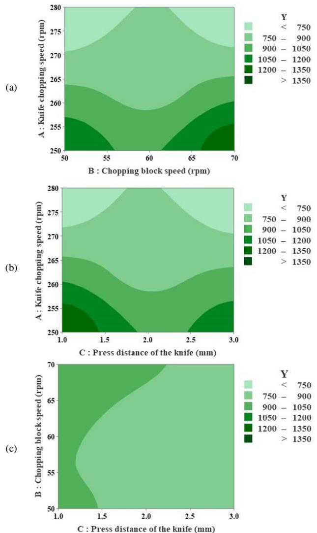
Fig. 6. 2D contour plots showing the effects of (a) A and B, (b) A and C, and (c) B and C on chopping time.
