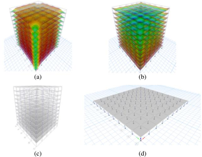
Fig. 1. ETABS software models: (a) with floating column, (b) without floating column, (c) short-span structure (5x6 m), (d) long-span structures (10x10 m).
