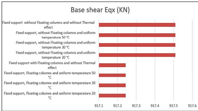
Fig. 2. Comparison of base shear in the x-direction.
