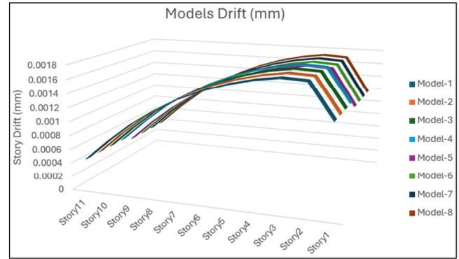
Fig. 3. Story drifts in the x-direction.
