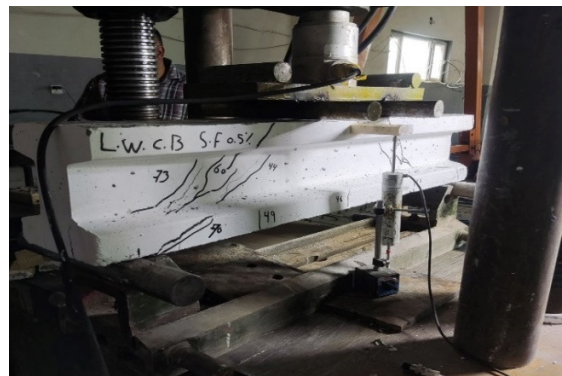
Fig. 4. The beam under the test device.
