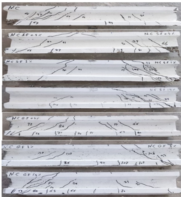
Fig. 11. Crack patterns for normal concrete group.
