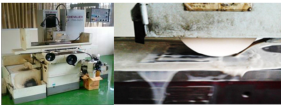
Fig. 1. The grinding machine of flat surface machining.
