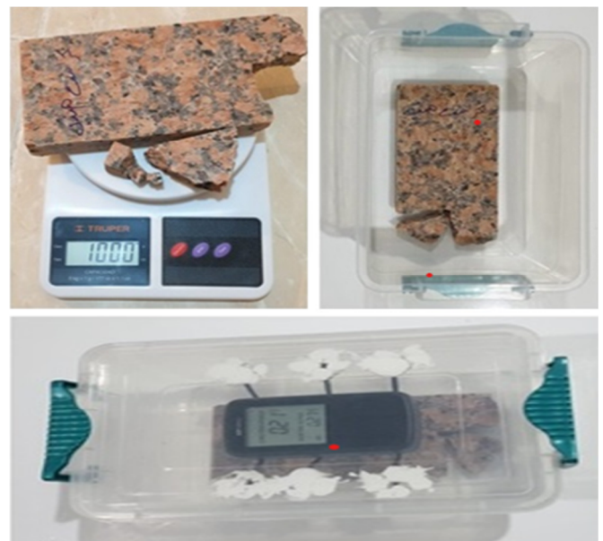
Fig. 1. Sample preparation and ^{222}\text{Rn} measurement process.
